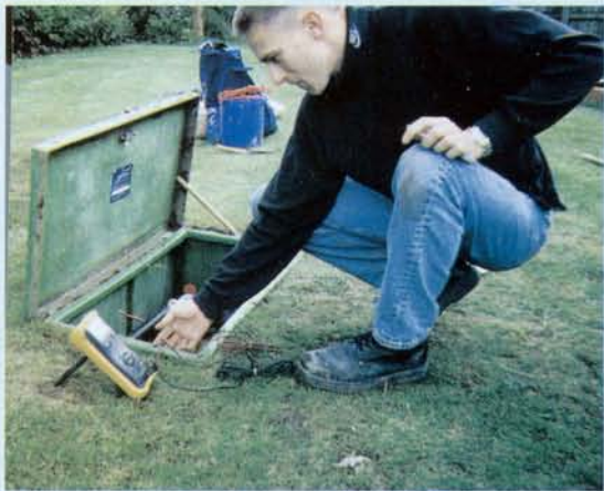
Monitoring an underground tank CP system
